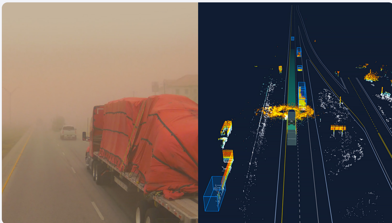
Launching driverless operations from Fort Worth to El Paso required validating behavior in dust storms — here our multi-modal sensor suite sees through dense dust at twice the range of cameras, highlighting the safety advantage of our sensor approach.
