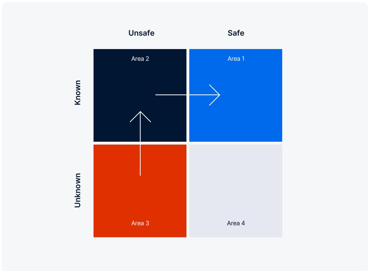
Figure. Scenario categories and the desired evolution derived from SOTIF analysis
