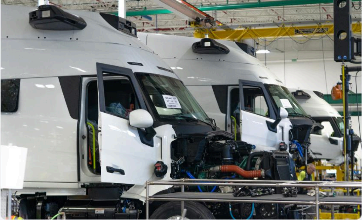
Lineside integration of the Aurora Driver hardware kit at Volvo's New River Valley, VA manufacturing facility
