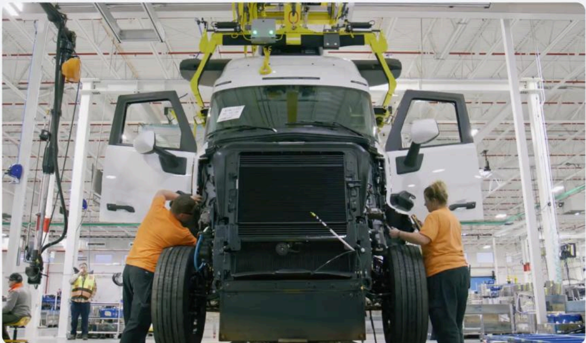
Lineside integration of the Aurora Driver hardware kit at Volvo's New River Valley, VA manufacturing facility
